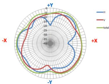
The antenna characteristics shows more or less circular radiation field. However using the device right on a notebook or other heavy device may partially degrade the signal significantly. Applying an USB-USB extender cable of min. 10 cm will always provide the best radio experience.
